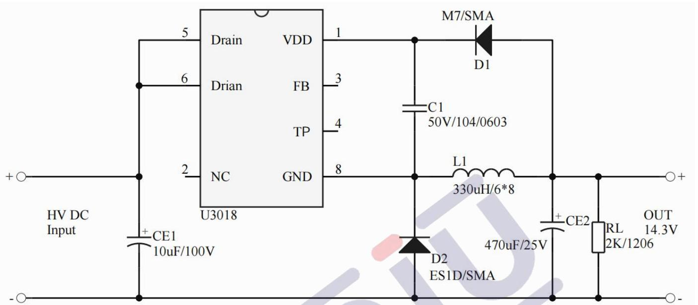
图-1 :  $V_{IN} > 30V, L = 330\mu$  ;  $HV_{IN} < 30V, L = 100\mu H$
